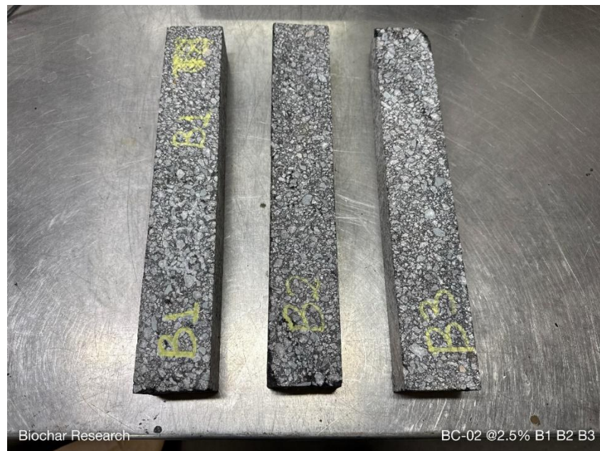
Figure 9-1: BC-2 2.5% Fatigue Beams B1 B2 and B3
