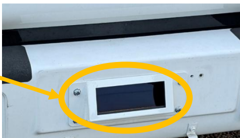
High-resolution LiDAR to detect small objects or lying people on the road ahead
