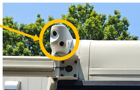
Front & rear side view camera
